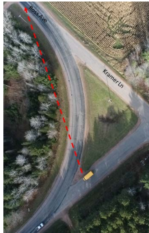
Figure 1: School Bus looking to turn westbound on Ross Ave. Note this is a slow accelerating vehicle and the sight line to ensure traffic heading south to westbound is difficult.
