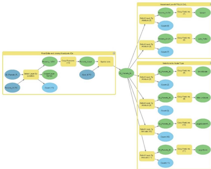
FIGURE A1-7: Model which Selected Vacant Parcels, Low IMPVL/LNDVL Parcels, and Potential Scale Based on Selection Criteria
